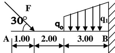
$$\begin{aligned} F &= 400 \text{ daN} \\ q_0 &= 50 \text{ daN/m} \\ q_1 &= 150 \text{ daN/m} \end{aligned}$$
