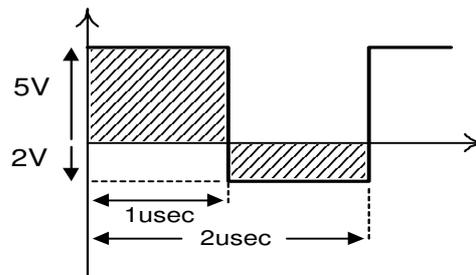
$$U_m = ((5V * 1\mu\text{sec}) - (2V * 1\mu\text{sec})) / 2\mu\text{sec} = 1,5 V$$
