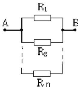
$$R_{AB} = \frac{1}{\frac{1}{R_1} + \frac{1}{R_2} + \dots + \frac{1}{R_n}}$$
